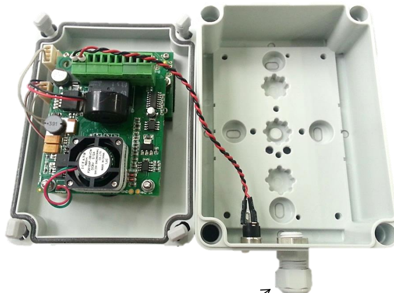
Cable gland for RS232 or RS485 connection
