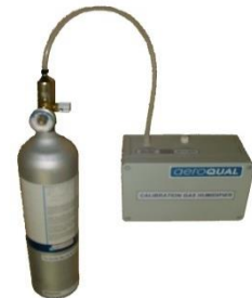
Zero air connected to R42
