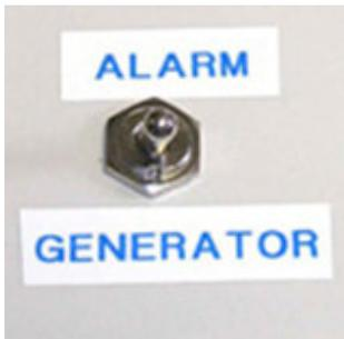
Use the toggle switch on the side of the R-25 Relay to select the operating mode desired (NO or NC State).
