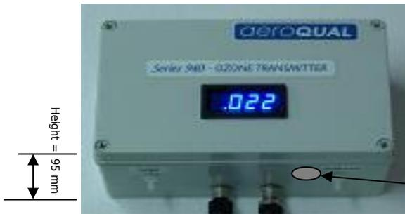
The S945 has a Temperature and RH probe located here
