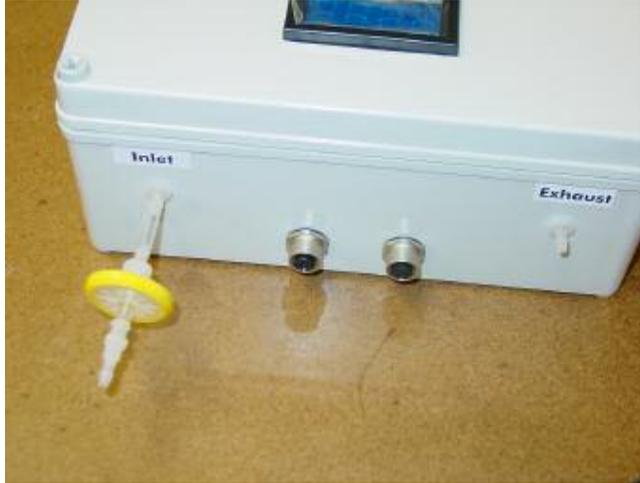
It is recommended that an inlet filter is installed at the entrance to any tubing to prevent contamination of the inlet tubing. Install inlet filter as shown. The filter should be a 5 micron pore size, PVDF or PTFE membrane filter, diameter at least 30 mm, hydrophobic. Sample tubing should be a maximum of 5 m in length and be inert PTFE, FEP or PFA tubing.
