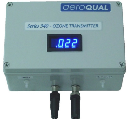
Series 940 Ozone Transmitter with LED display
