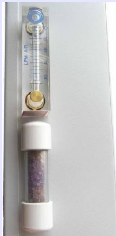
Image shows the flowmeter (top) & dry air indicator (bottom). Indicator turns from dark blue to purple when the desiccant requires replacement.
