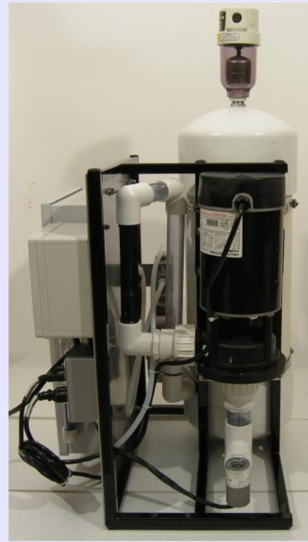
View of the OSW-3 from the inlet side. The injector and plumbing is viewed from this side very well.
