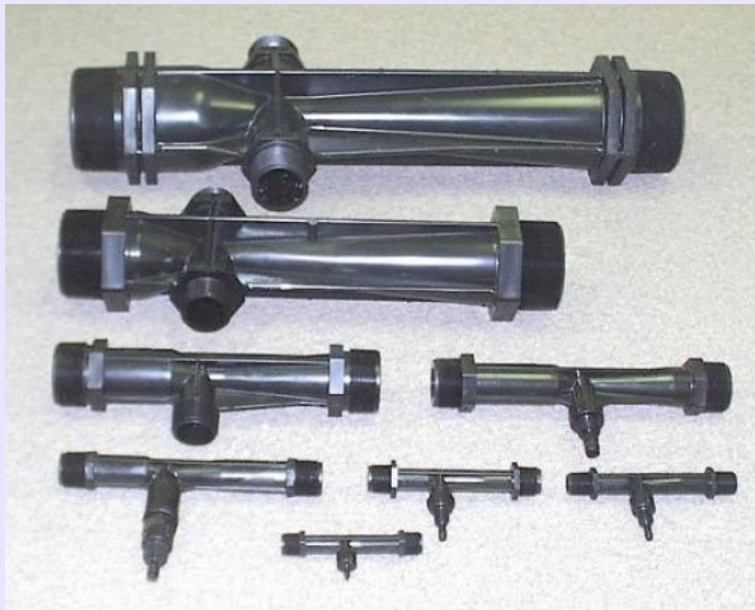
Image shows the various sizes of ozone injectors & ozone venturis. Injectors range from 1/2-in MPT to 4-in MPT process connections. All ozone injectors made from high quality black Kynar (PVDF).
